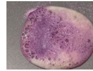
2) Foaming indicates neutralization in process
