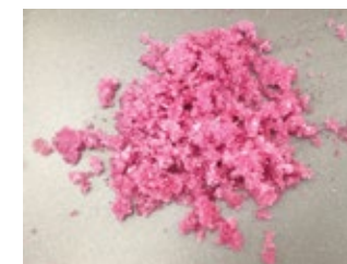
4) Spilled liquid has been neutralized & absorbed
